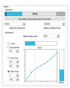
Few simulator softwares has built in brake force limiter, which works similar to our Brake output limit setting. It is recommended to disable them by setting it to 100% (also all pedal manipulation features).
