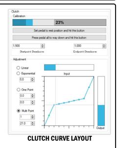
Multi Point curve setting is selected, the input and output signal are coupled by the curve.
