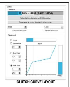
Multi Point curve setting is selected, the input and output signal are coupled by the curve.
