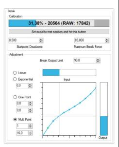
Few simulator softwares has built in brake force limiter, which works similar to our Brake output limit setting. It is recommended to disable them by setting it to 100% (also all pedal manipulation features).
